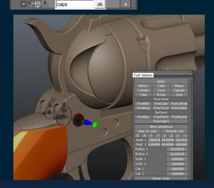
Select the clone function and switch to the rectangular marquee then select the screw you have created, a new cloned version will appear, move this into the position of the other screws in the reference. Once you have created the trigger screw and the bolt screw and ejector tube screws, move onto the backstrap screws and rear guard screws; inset these last sets quite deeply.
